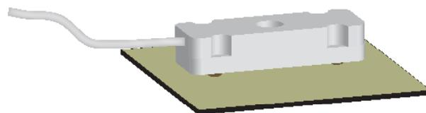
*When mounted in a metal tray, mount the sensor face down on an insulating surface such as a vinyl floor tile. Secure the sensor with tie wraps or wooden brackets.*
