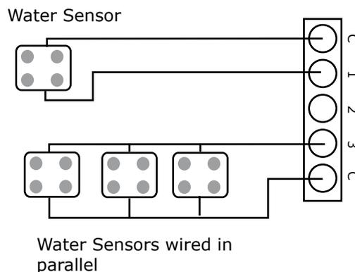
*Connect the sensors to the C123C block. "C" is common (ground). If more than three water sensors are to be used, they can be wired in parallel (not series). When wired in parallel, when any sensor becomes wet it will trip the alarm for that input.*
