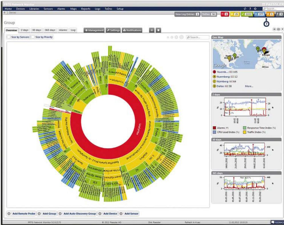
The sunburst view diagram allows a quick overview of the complete status of the monitored devices. The inner ring represents the entire network. If this ring is red, this indicates that a device in one of the outer rings is showing a failure.
